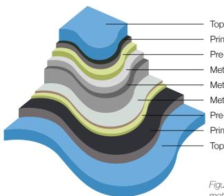
surface quality white products for the domestic appliance market to brightly coloured, long-lasting products for construction applications. Prepainted metal products are generally referred to by their topcoat and while the focus of this document is mainly on the varieties of topcoat, it is important to remember that the other layers also contribute to the final product performance.
